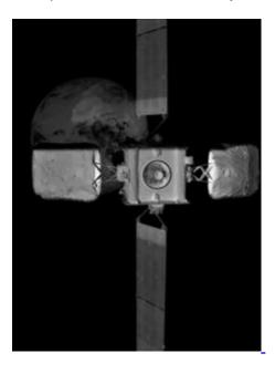
An image of Intelsat 10-02 taken by MEV-2's infrared wide field of view camera at 15m away. Photo credit: Northrop Grumman
